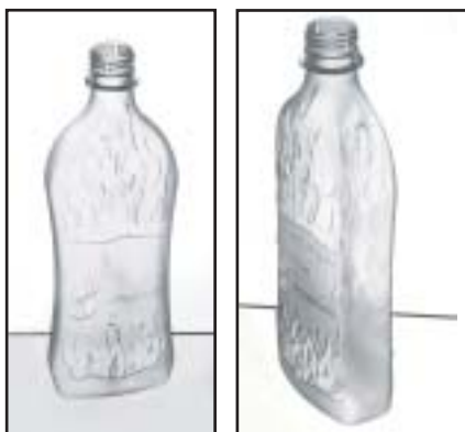
Magplastic hipflask bottle with preferential heating
